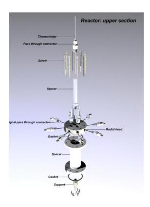
gas tight electrical connections made by modified mini spark plugs (NGK: 5812 CM-6, Japan)
